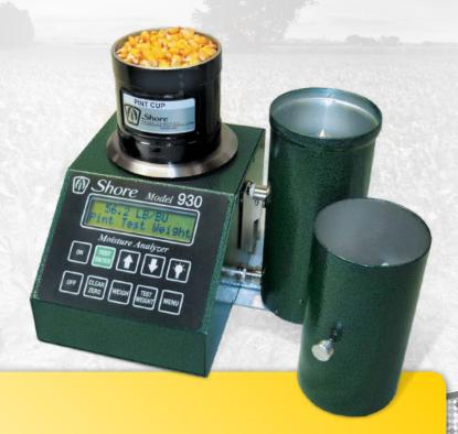
The Shore Model 930 Moisture Tester delivers quick, accurate results when testing a multitude of commodities. Featuring an integrated scale and moisture tester, the Model 930 helps verify moisture content of grain before going to market, without the need for moisture or temperature conversion tables.
