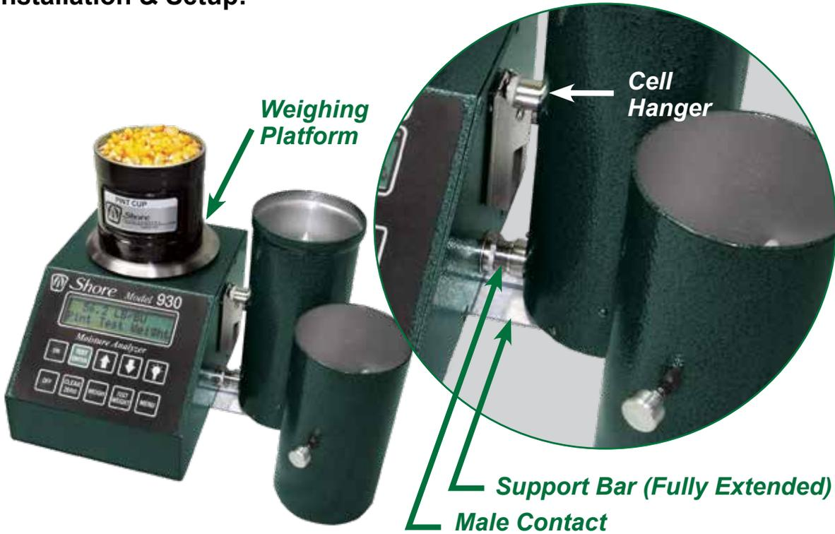
1. Loosen the two thumbscrews holding the console support bar to the bottom of the console. Slide the support all the way out and lock in place by re-tightening the thumbscrews.
